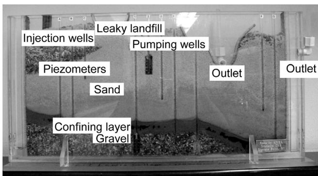
**Figure 1. Groundwater model used in the groundwater lab.**
